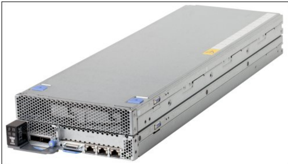
Figure 6. NeXtScale Storage Native Expansion Tray attached to an nx360 M4 compute node
