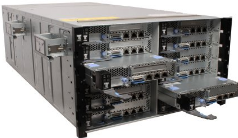
Figure 1. Twelve NeXtScale nx360 M4 servers that are installed in an NeXtScale n1200 enclosure
