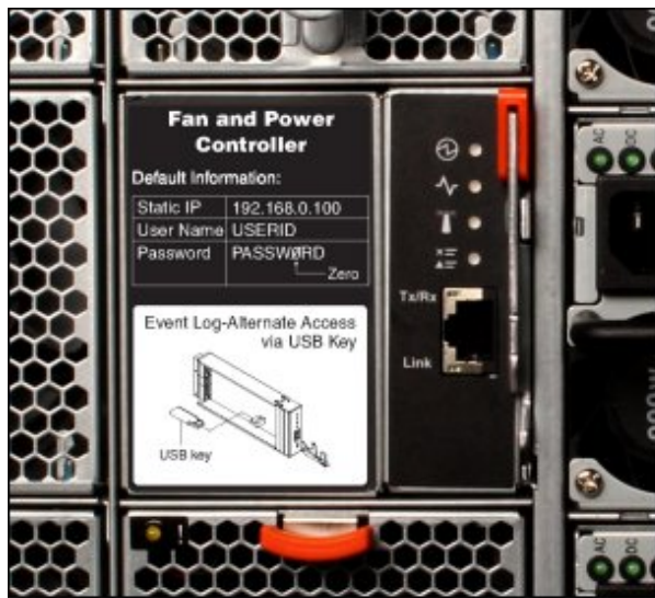
Figure 12. Fan and Power Controller
