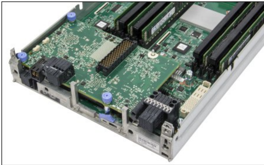
Figure 2. The adapter installed in the Flex System x222 Compute Node
