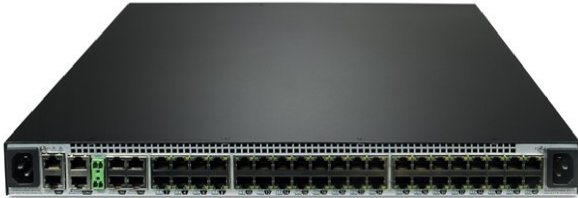
Figure 2. Ports at the rear of the Avocent Universal Management Gateway 6000 for IBM
