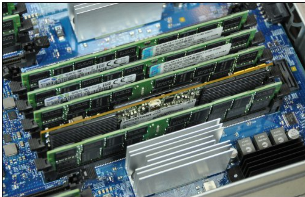
Figure 5. eXFlash DIMM installed in the Compute Book
