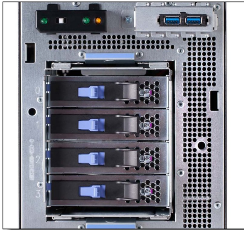
Figure 6. Simple-swap drive bays of the compact tower models (accessible with the front bezel removed)
