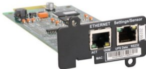
Figure 2. UPS Network Management Card
