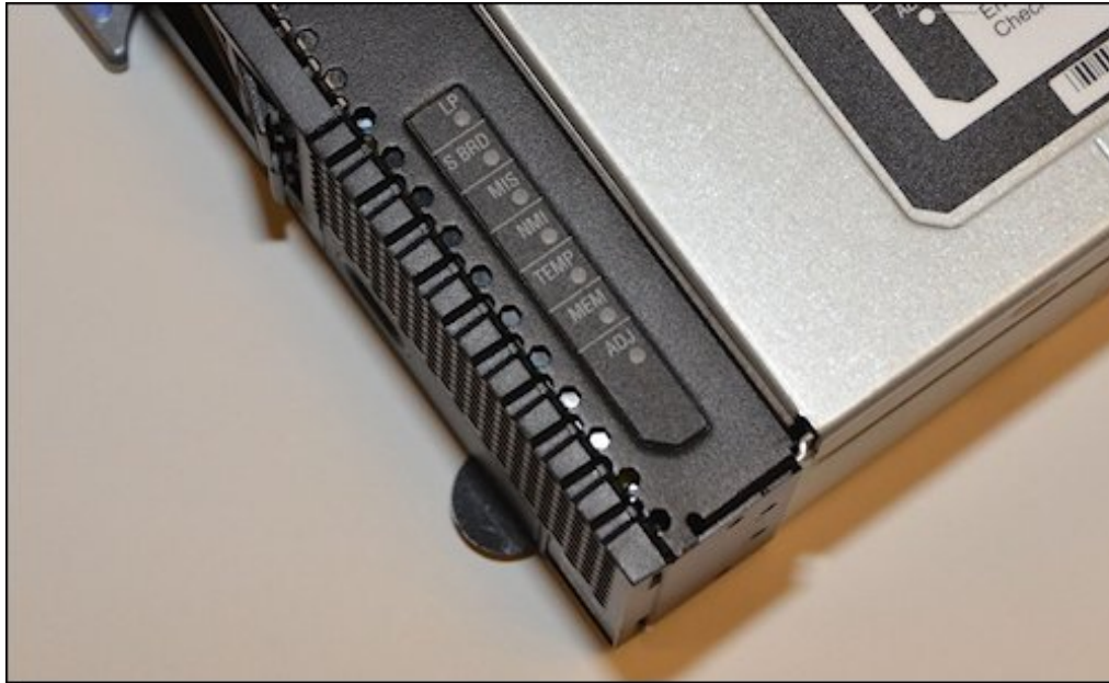
Figure 10. Location of x240 light path diagnostics panel
