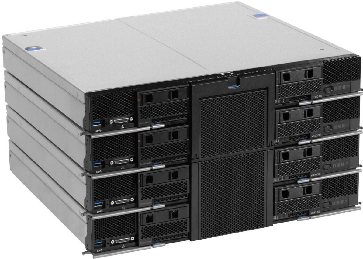
Figure 4. Four x880 X6 Compute Nodes in an 8-socket complex
