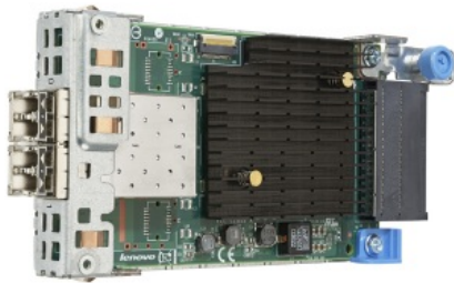
Figure 4. ThinkServer LPm16002-M6-L AnyFabric 16Gb 2 Port Fibre Channel Adapter by Emulex
